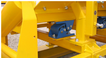
Conveyor impact table designed with ROSTA ESL ®
