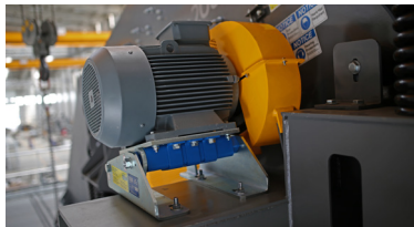
Fixed plant vibrating screen drive designed with ROSTA MB ®
