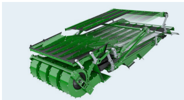
Cleaning shoe for combine designed with ROSTA AS ®
